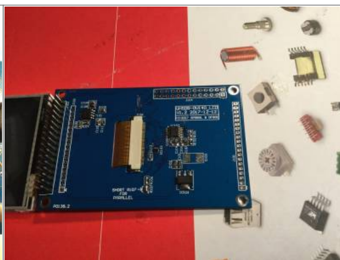
OVI40 3.5,, display, component side (photo:DL8EBD)
