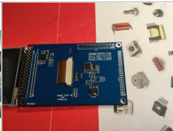
OVI40 3.5" display, component side (photo:DL8EBD)
