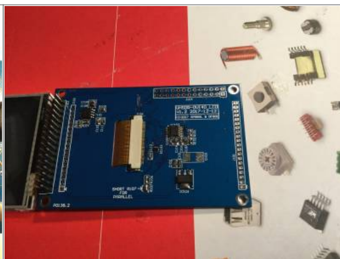
OVI40 3.5,, display, component side (photo:DL8EBD)
