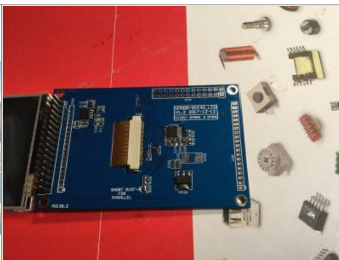
OVI40 3.5" display, component side (photo:DL8EBD)
