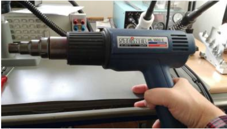
Hot air pistol used for de-soldering - see text
