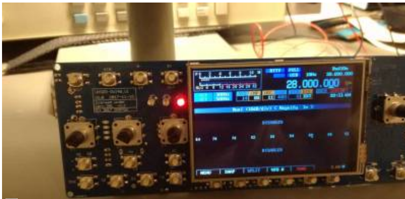
OVI40 UI and display board (photo DF9EH)
