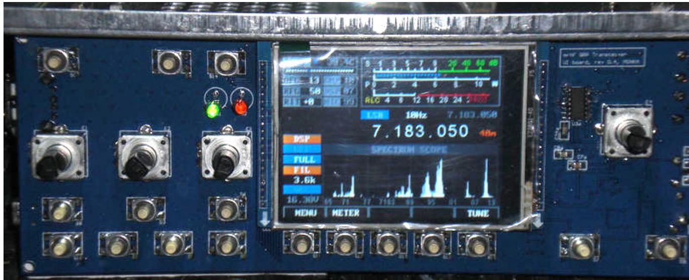
SDR technology (software defined radio) enables a completely new “feel” on the radio. The symbiosis of modern digital technology and analogue transceiver technology is the same, QRM/QRN is not exclusive to old iron!
