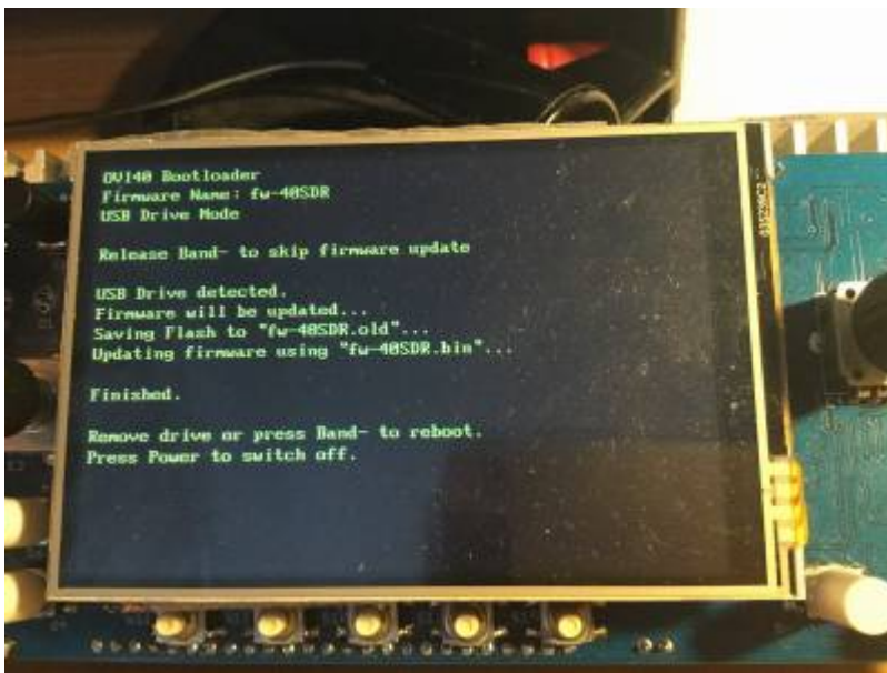
Boot loader upgrade with USB stick (photo DL8EBD)
