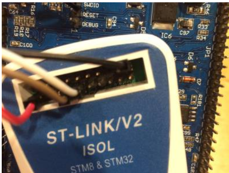
Connection ST-Link to UI board (photo F4HTX)
