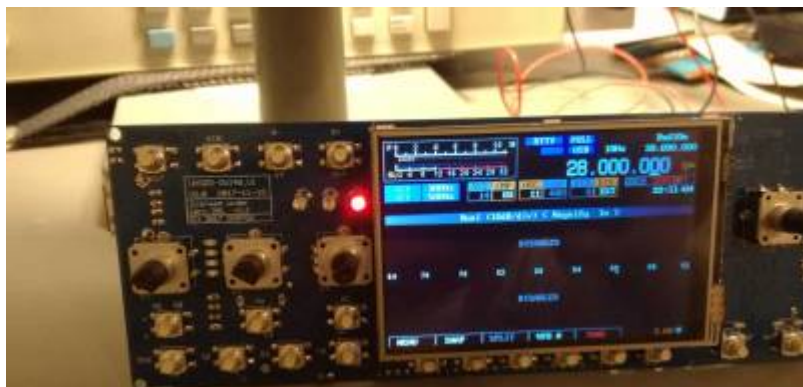
OVI40 UI and display board (photo DF9EH)
