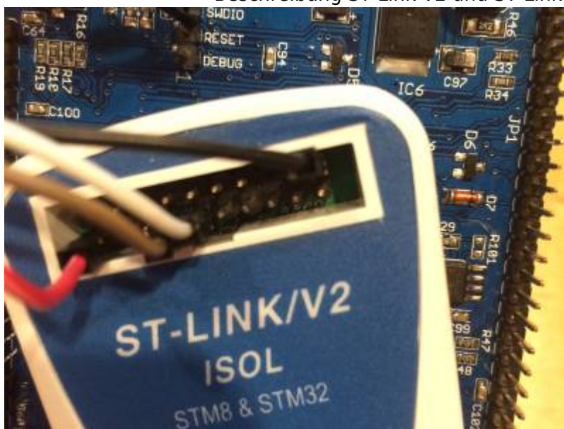
Connection ST-Link to UI board (photo F4HTX)
