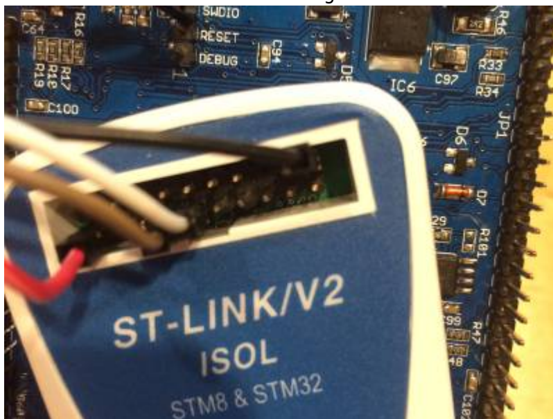
Connection ST-Link to UI board (photo F4HTX)
