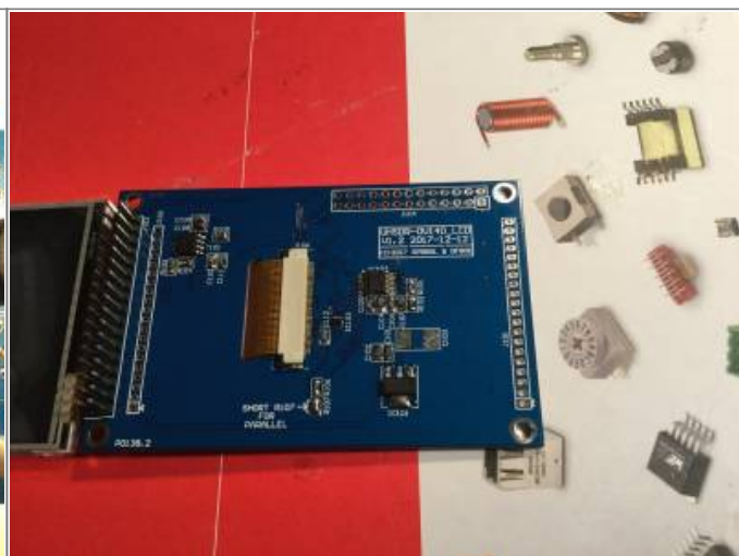
OVI40 3.5,, display, component side (photo:DL8EBD)
