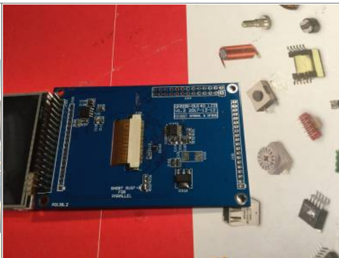
OVI40 3.5,, display, component side (photo:DL8EBD)
