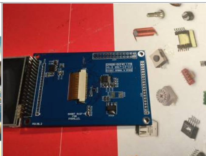
OVI40 3.5,, display, component side (photo:DL8EBD)
