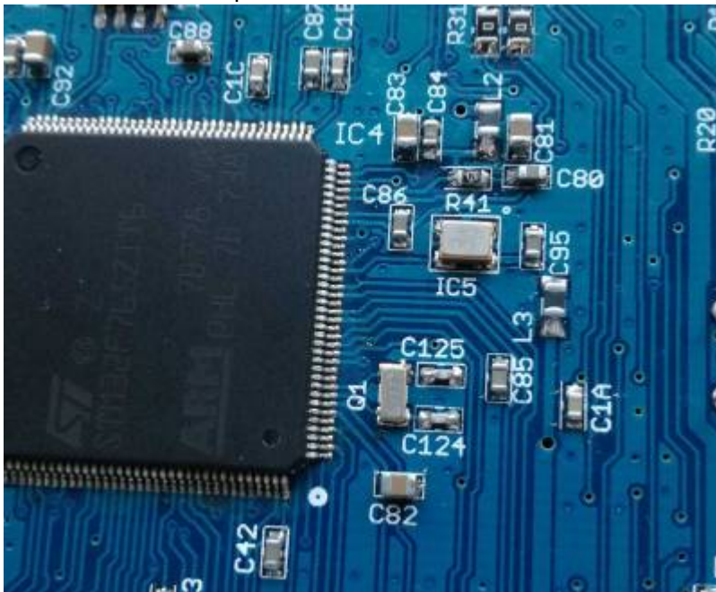
Orientation of TXCO & MCU (photo DF9EH)
