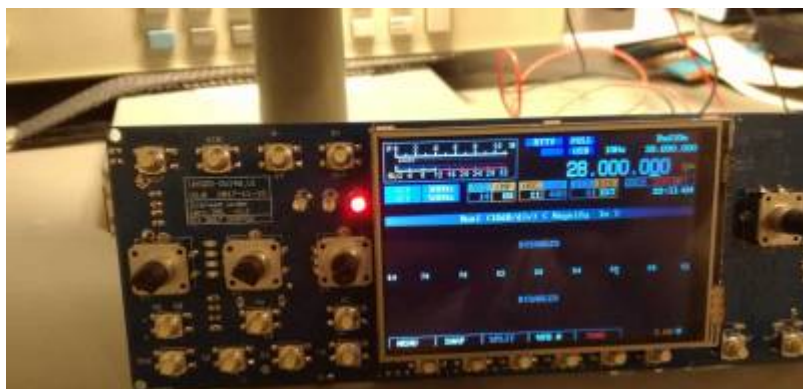
OVI40 UI and display board (photo DF9EH)
