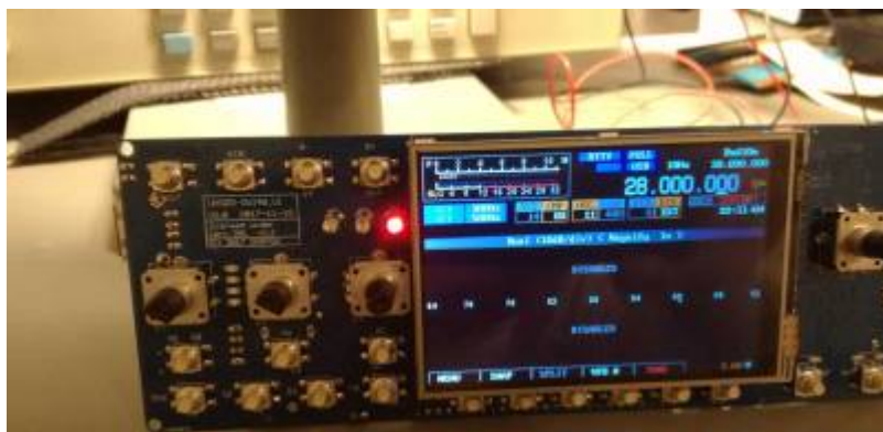
OVI40 UI and display board (photo DF9EH)
