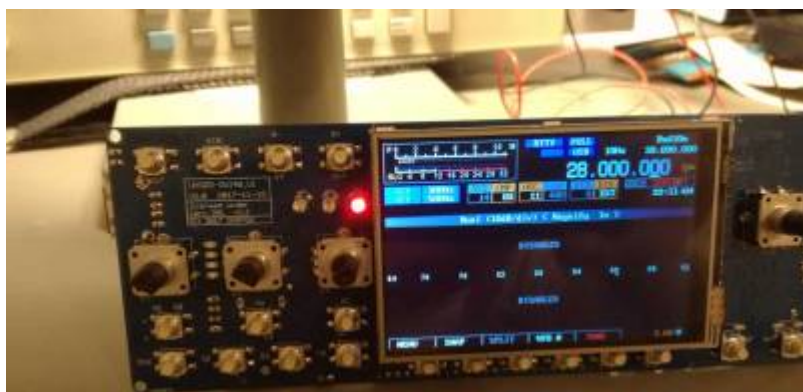
OVI40 UI and display board (photo DF9EH)
