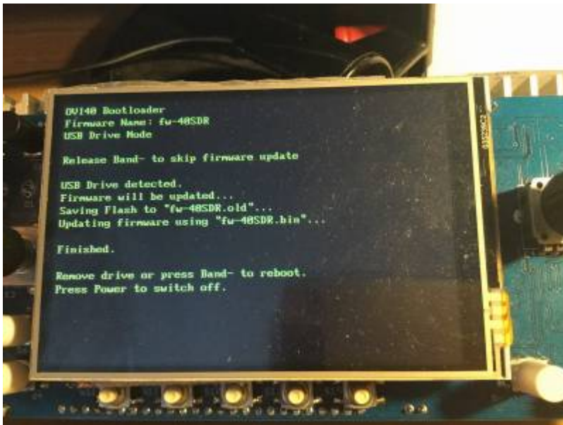
Bootloader Upgrade per USB Stick (Photo DL8EBD)
