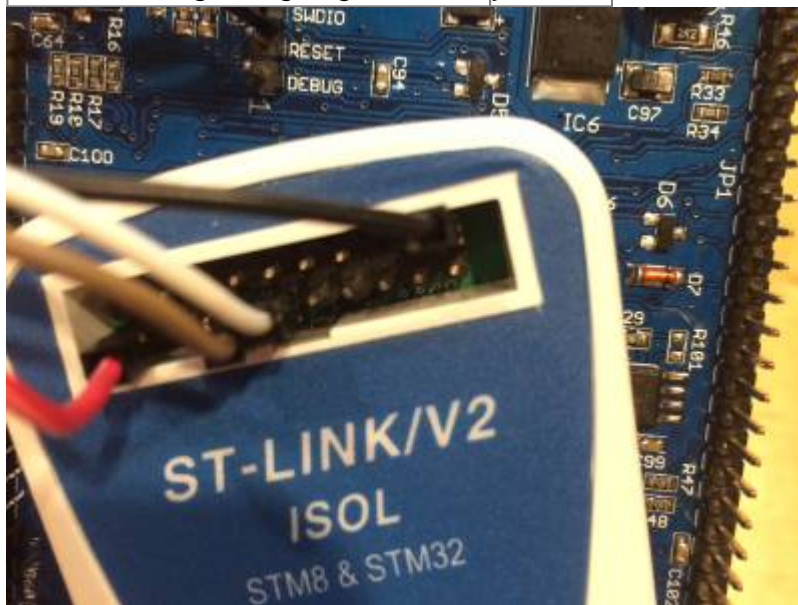
Connection ST-Link to UI board (photo F4HTX)
