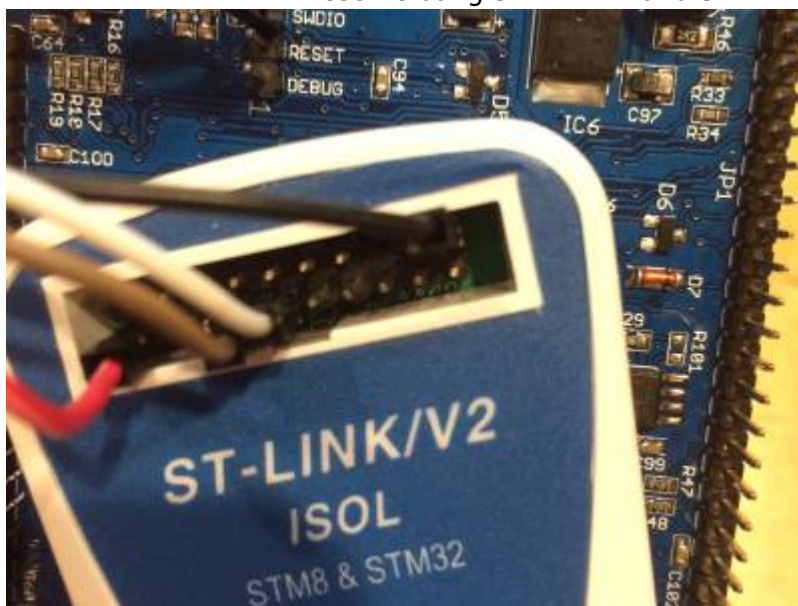
Connection ST-Link to UI board (photo F4HTX)
