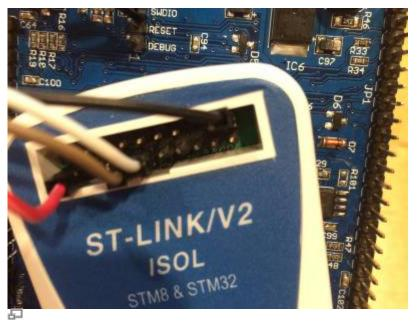
Connection ST-Link to UI board (photo F4HTX)
