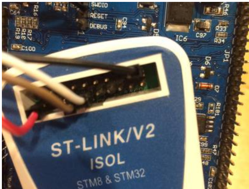
Connection ST-Link to UI board (photo F4HTX)
